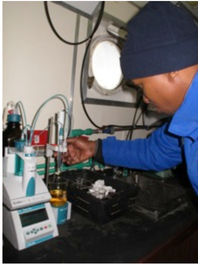
Figure 1: Preparation of dissolved oxygen Auto-titrator by Mbulelo Makhetha (DEA). Photo: B. Hölscher
