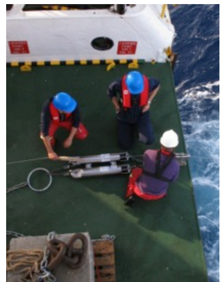
Figure 6: Acoustic release deployment by mooring technicians. Photo: B. Hölscher
