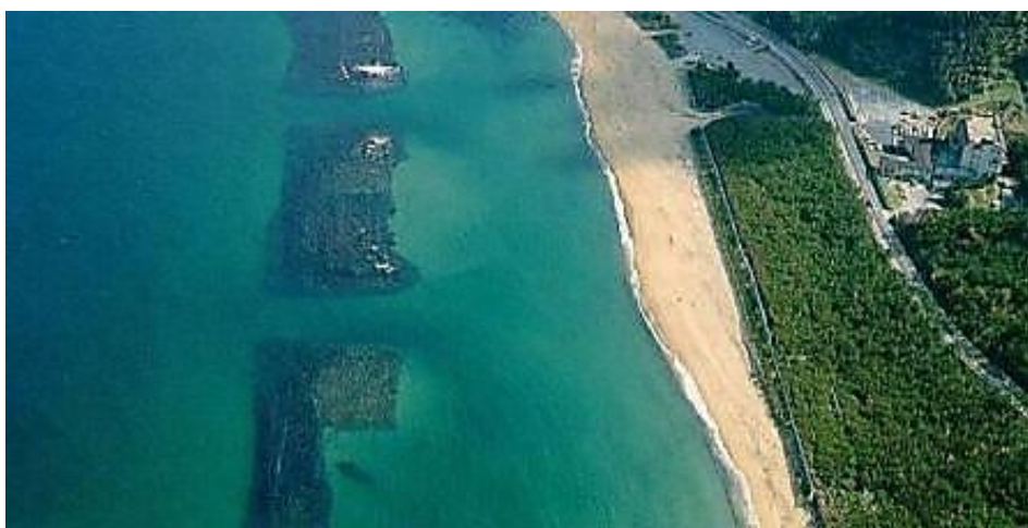
Figure 10: Example of beach accretion through submerged artificial reefs
