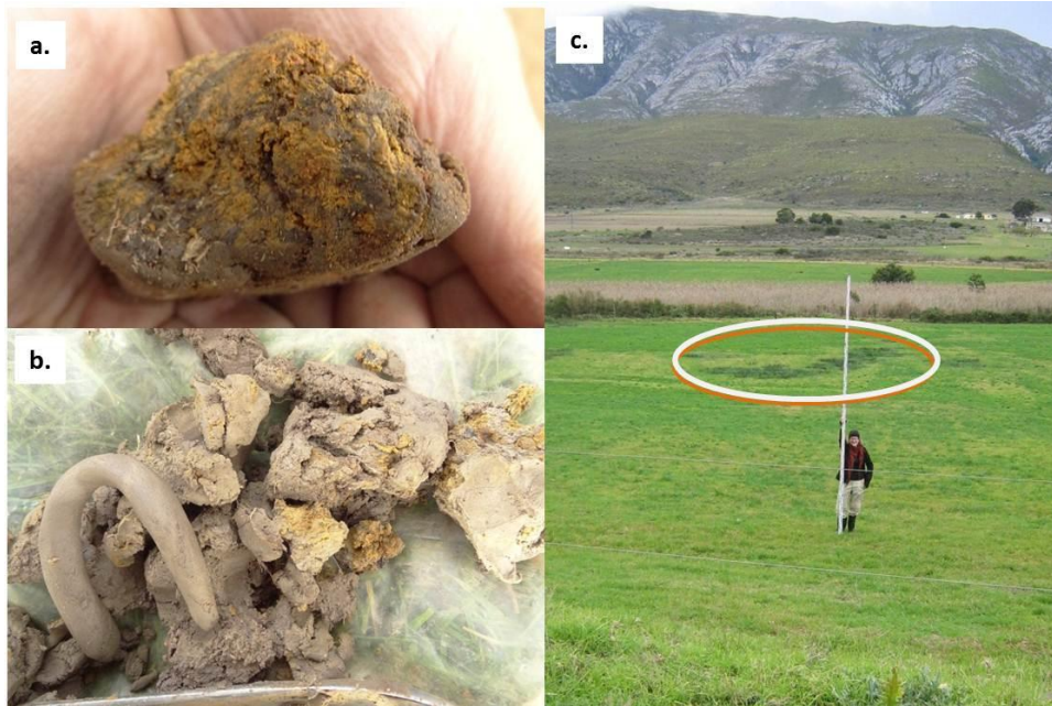
Figure 34: Indicators of soil wetness used in wetland delineation (a.) and (b.) showing mottling and gley of the plinthic B horizon due to the fluctuation of water table. (c.) The red circle indicates the location of sedge vegetation within the pasture along the right side of Transect 3. (Photo by Author)
