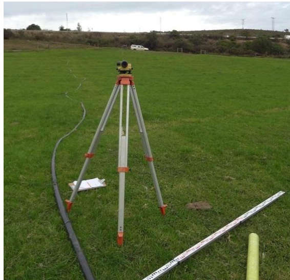
Photo 10: The surveyor’s level and the leveling staff (Photo by Lieke Jager)
