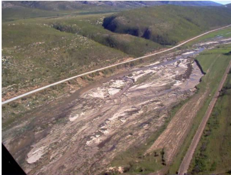
Figure 3.8: An aerial photograph taken from a helicopter of the main floodplain of the Kromme River after a large flood event. The floodplain was once covered by palmiet wetlands, specially adapted to withstand the force of the flood waters. The removal of the palmiet wetlands has destabilized the system, causing massive headcuts and lateral erosion which lowered the water table and reduced the agricultural potential of the land.
